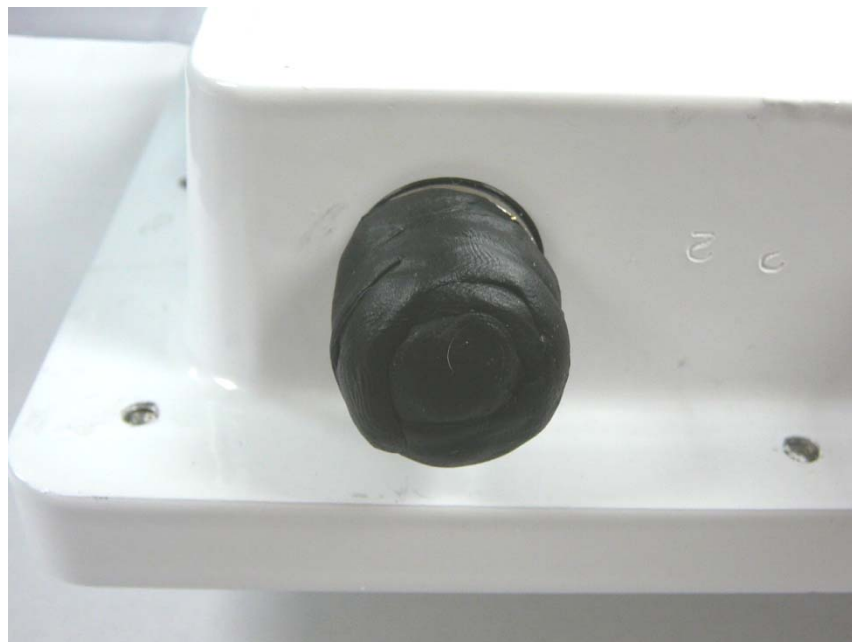
Figure 2: Properly Taped External Antenna Port.
